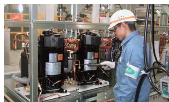
Compressor also developed and manufactured by Mitsubishi Electric* Refrigerant leak inspection process using helium gas
